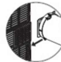
3. Insert the other end of the exhaust hose into the hole in the window slider kit.
